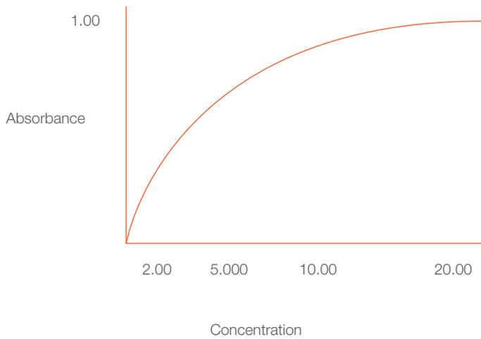
It can be seen that we can determine the concentration by measuring the absorbance at the lower levels, but any slight change in absorbance can make a big difference in concentration at the higher levels.
